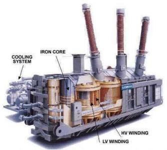
PART CROSS SECTION OF A VERY LARGE TRANSFORMER
