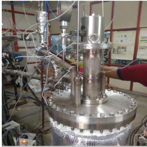
Fig 10.2 Testing of Level Sensor in Pb-Li test facility at IPR, Ahmedabad
