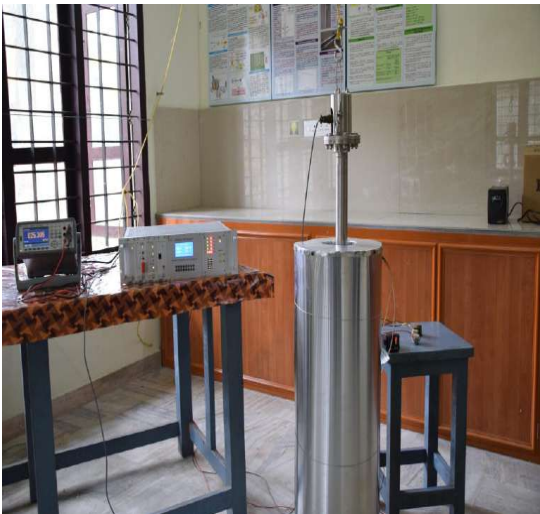
Level Probe testing setup with SS Blocks at VJCET
