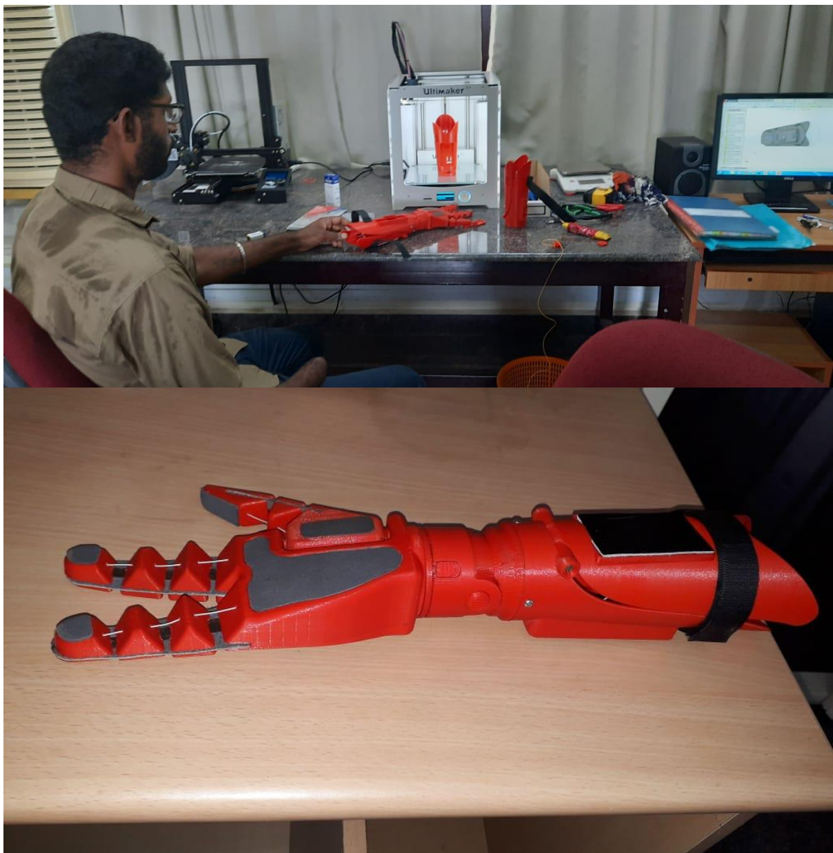
Powered Prosthesis Arm Developed at VJCET FABLAB
