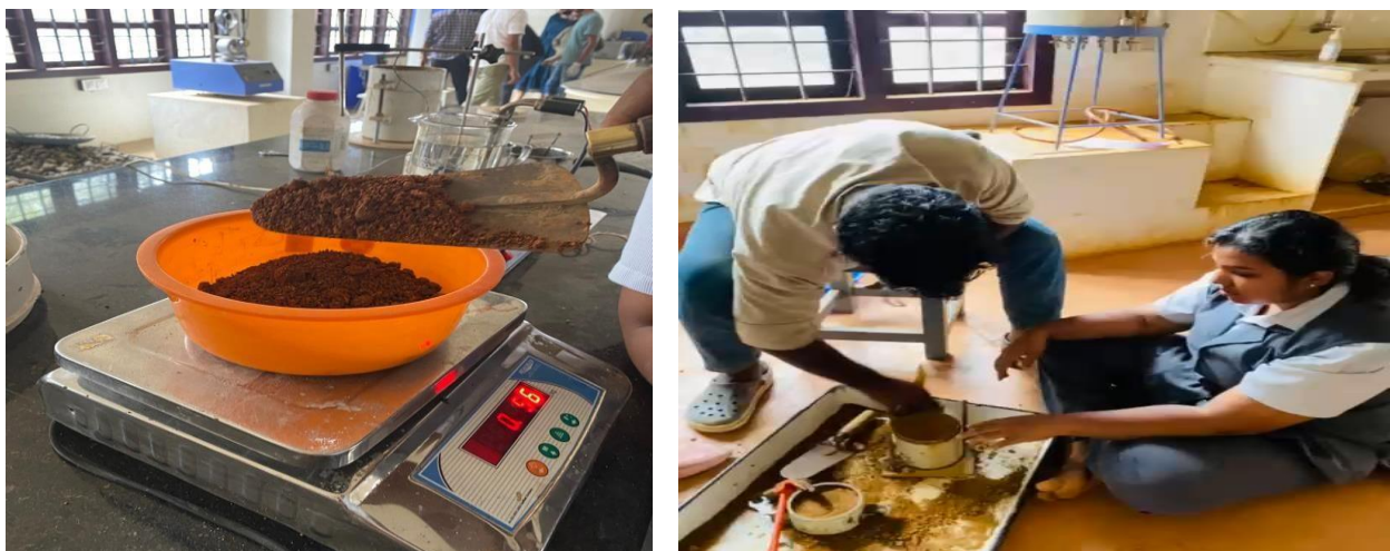
Fig 5.4: Standard Proctor test (self taken)
