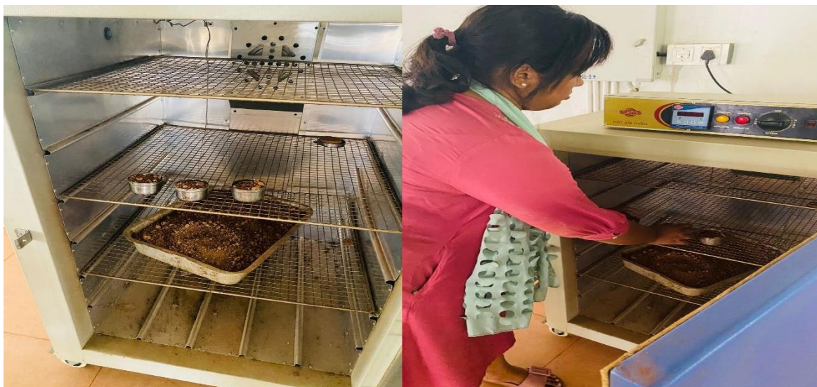
Fig 5.1: Water content determination (Self taken)
