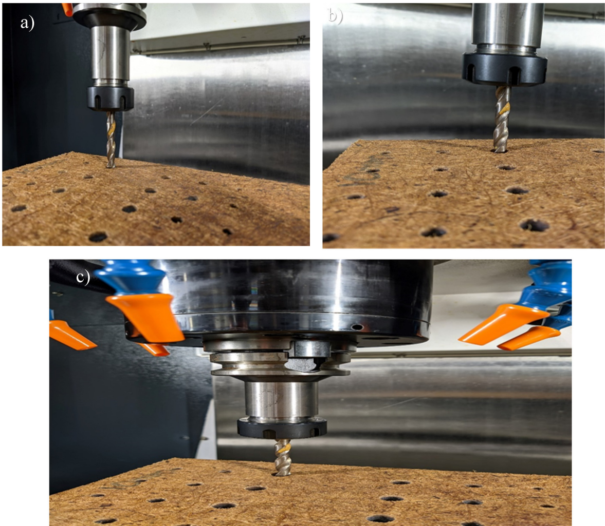
Fig. 1. CNC Drilling of CFRC a) 6 mm drill bit diameter. b) 8 mm drill bit diameter. c) 10 mm dill bit diameter.
