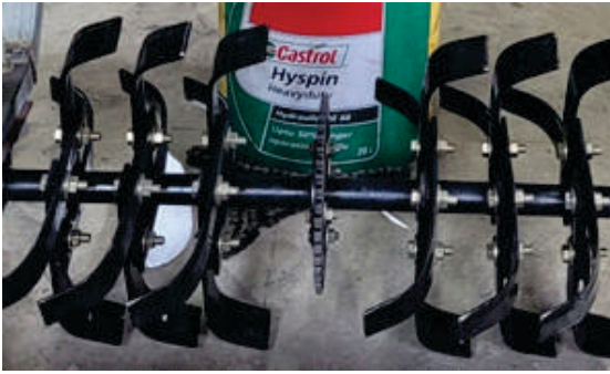
Fig. 8: Tilling Blades attachment
