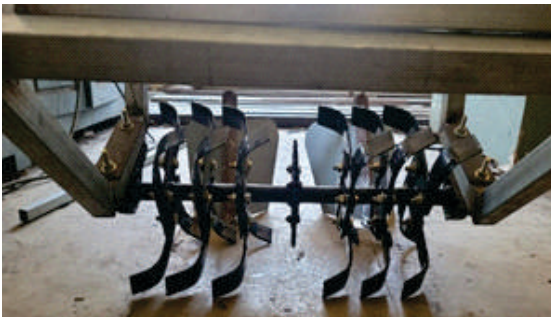
Fig. 9: Main shaft attachment to the main frame
