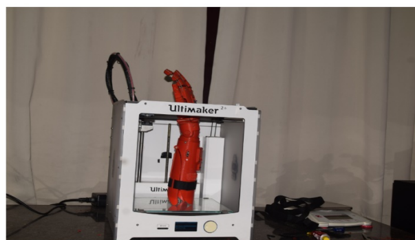
Fig. 3: Ultimaker 2+ Connect single nozzle 3D printer
