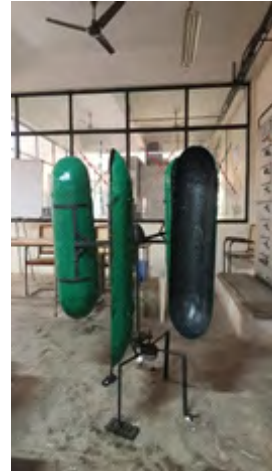
Fig. 8: Finished vertical axis wind turbine
